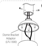
Insert the Dome Bracket Adaptor to 1.5" NPT screwthread (female) pipe or to the Wall/Ceiling/Parapet Mount Adaptor (LBK1000W/LBK1000P/LBK1000R) and tighten the three pipe screws.
